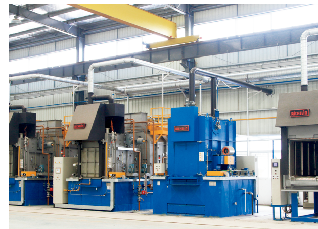
AICHELIN 热处理生产线 ACHELIN Heat Treatment Production Line
