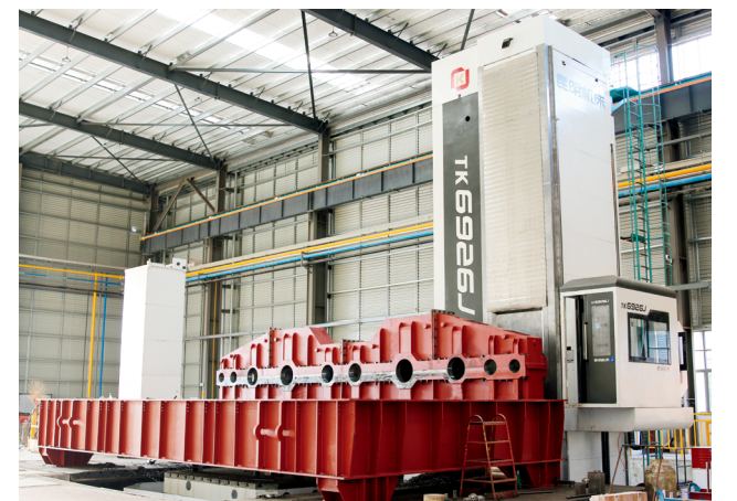
TK6926 数控刨台镗床 TK6926 CNC Planer Boring Machine
