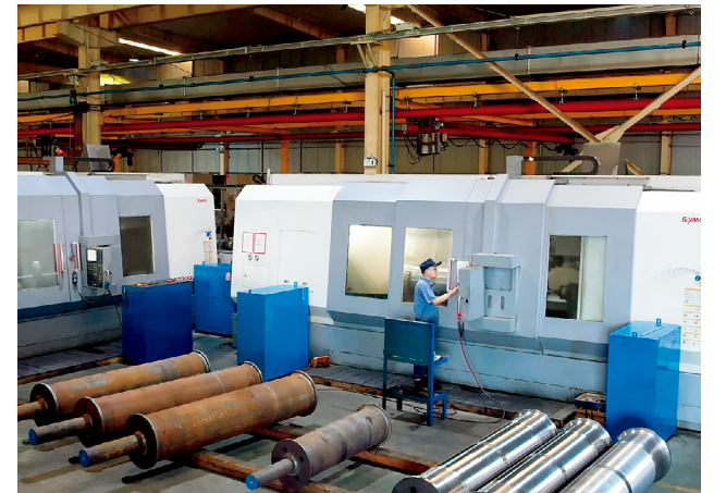
HTC63300t 全功能斜床身数控车床 HTC63300t Full-function CNC Lathe with Inclined Bed
