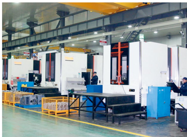
MAZAK 卧式加工中心 MAZAK horizontal machining center from Japan
